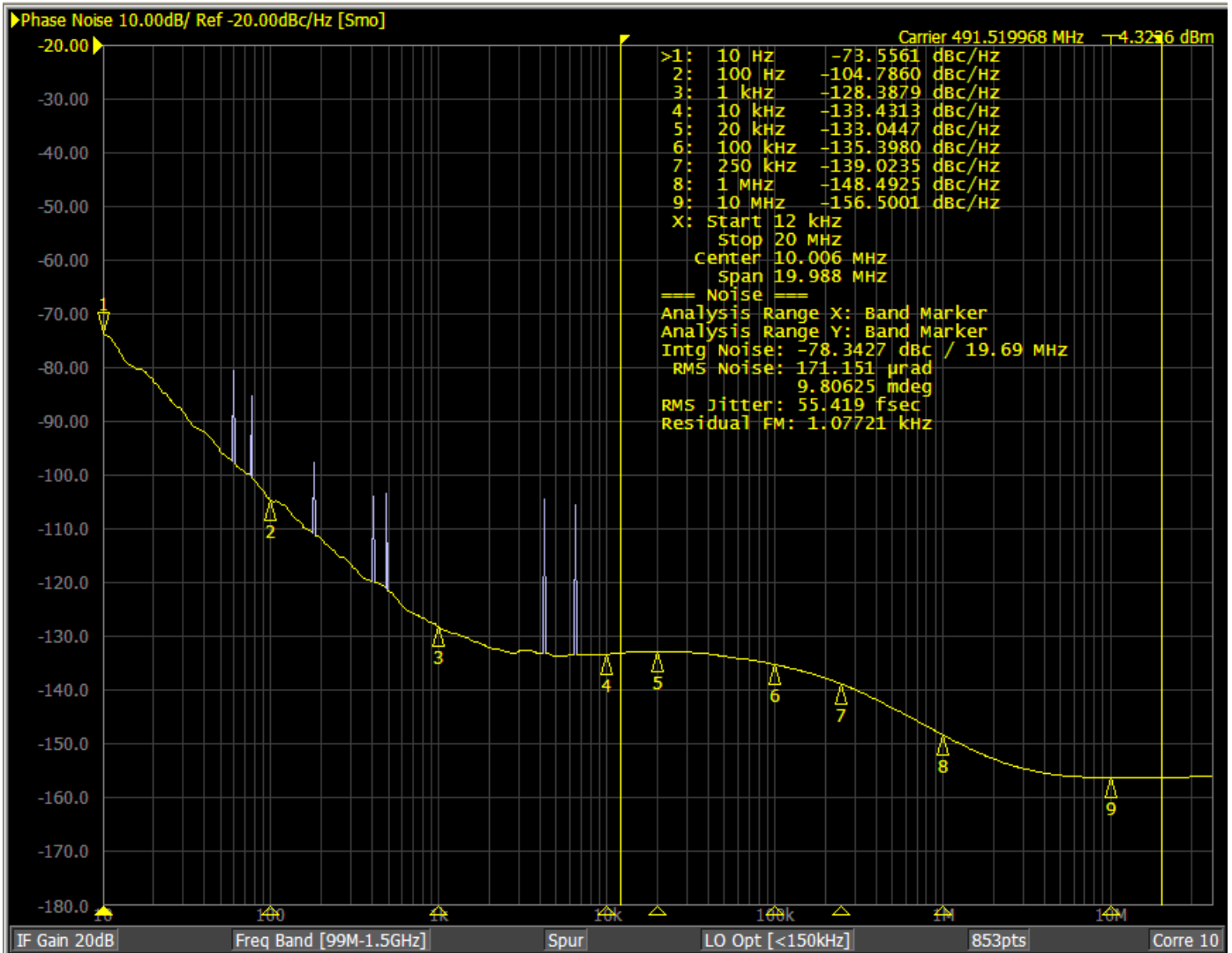
Figure 9. 491.52MHz Output Phase Noise
