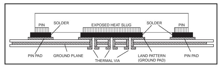
Figure 18: P.C. Assembly for Exposed Pad Thermal Release Path - Side View (drawing not to scale)
