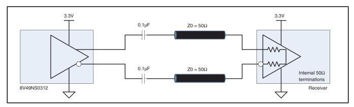
Figure 15: AC Termination for LVDS outputs used with an Input Clock Receiver with Internal 50 $\Omega$  Terminations and DC Bias.
