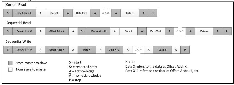
Figure 2: I<sup>2</sup>C Slave Read and Write Cycle Sequencing
