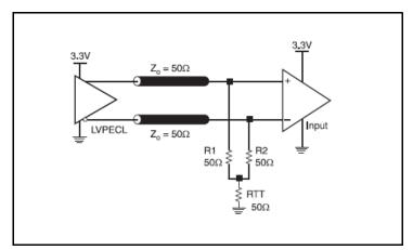
Figure 16: 3.3V LVPECL Output Termination
