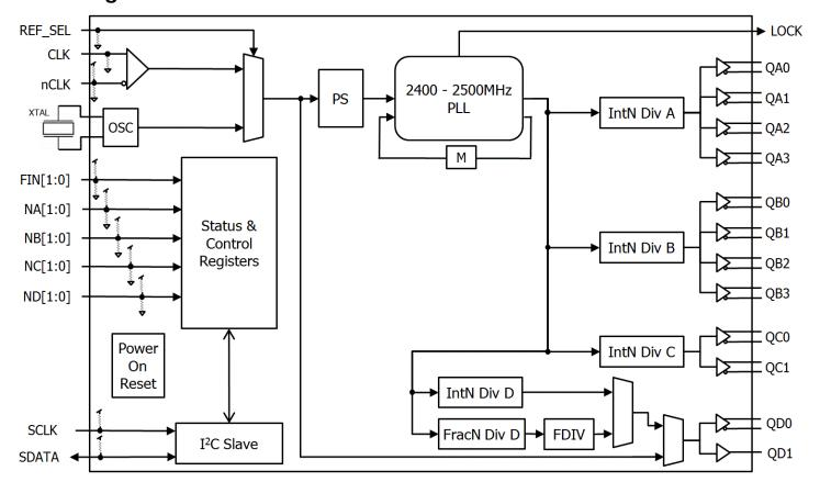
Figure 1: 8V49NS0312 Block Diagram
