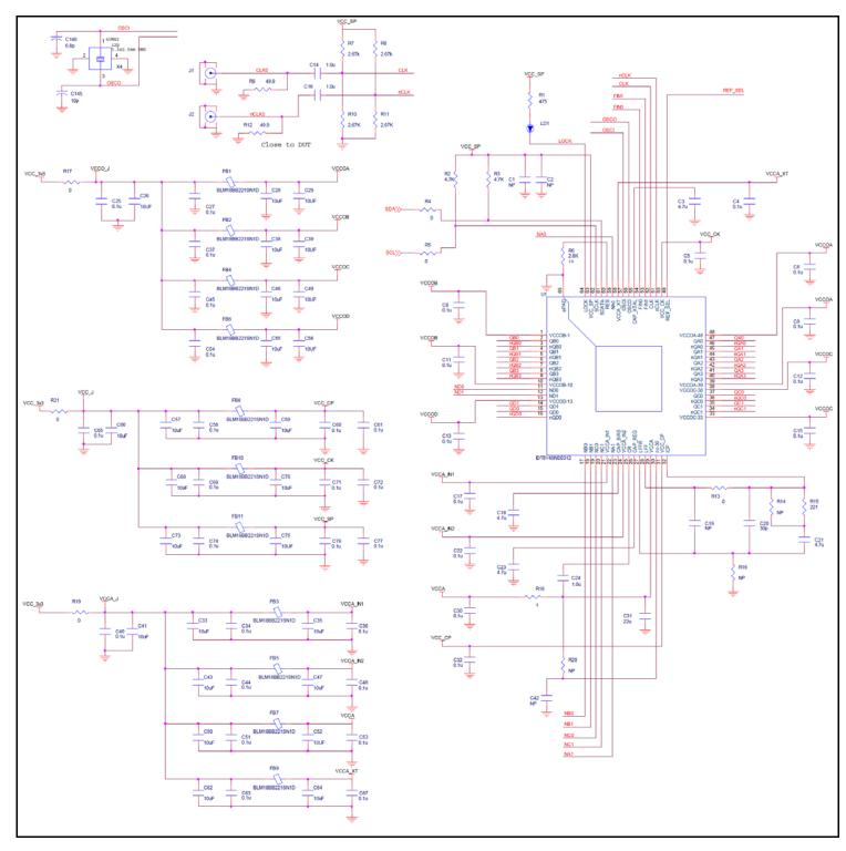
Figure 19: 8V49NS0312 Application Schematic
