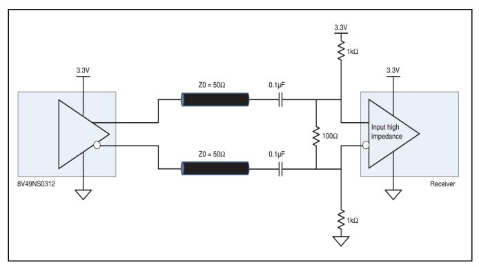
Figure 14: AC Termination for LVDS Outputs
