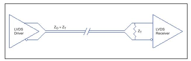
Figure 11: Standard LVDS Termination
