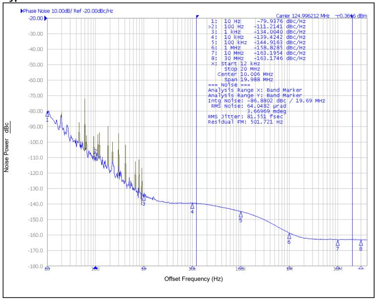
a. Measured using a 50MHz, 12pF crystal as input reference. The following loop filter components were used:  $R_Z$  = 150 $\Omega$ ,  $C_Z$  = 0.1 $\mu$ F, CP = 200pF. PLL Charge Pump Current Control set at 6.4mA.
