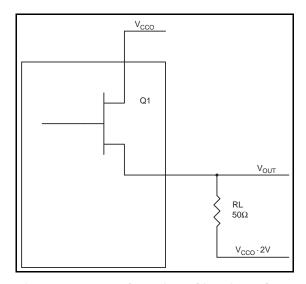
Figure 20: LVPECL Driver Circuit and Termination
