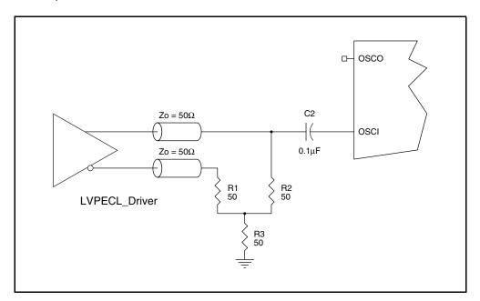
Figure 4: General Diagram for LVPECL Driver to XTAL Input Interface
