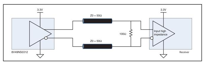
Figure 13: DC Termination for LVDS Outputs
