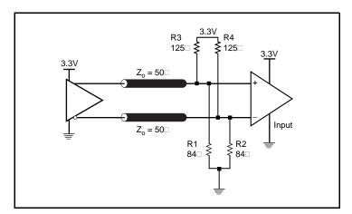
Figure 17: 3.3V LVPECL Output Termination
