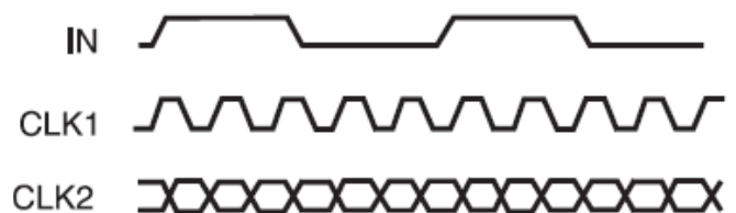
Input and Output Clock Waveforms with CLK1 Connected to FBIN
