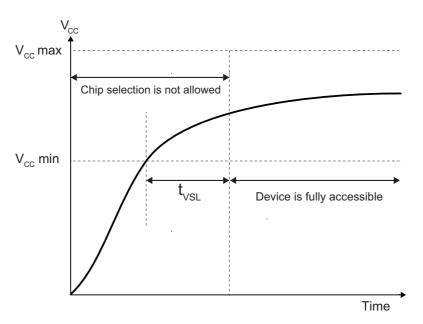
Figure 42. Power-Up Timing and Voltage
