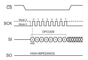
Figure 24. Write Enable Timing
