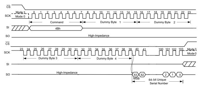
Figure 27. Read Unique ID Timing (SPI Mode)
