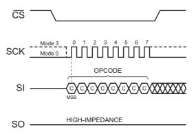
Figure 21. Chip Erase Timing
