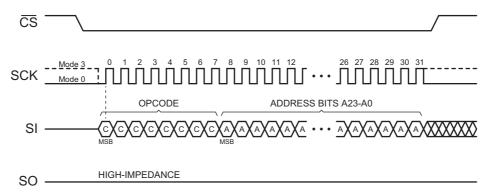
Figure 20. Block Erase Timing
