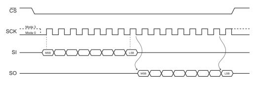
Figure 4. SPI Mode 0 and 3
