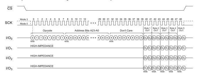
Figure 10. Quad-Output Fast Read Array
