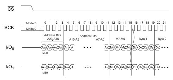
Figure 9. Dual-I/O Fast Read Array (Previous command set M5, M4 = 1,0)
