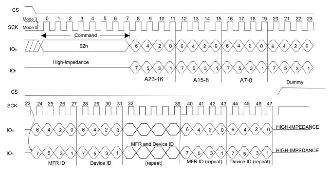
Figure 37. Dual I/O Read Manufacture ID/ Device ID Timing
