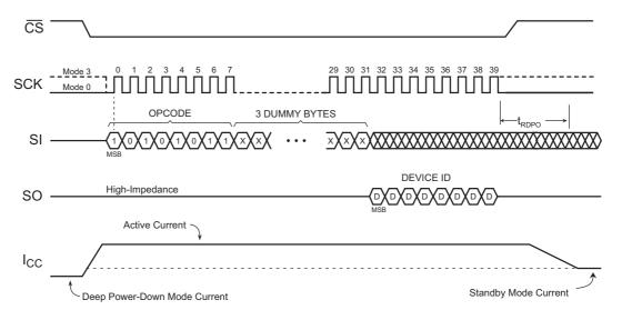
Figure 41. Resume from Deep Power-Down and Read Device ID Timing
