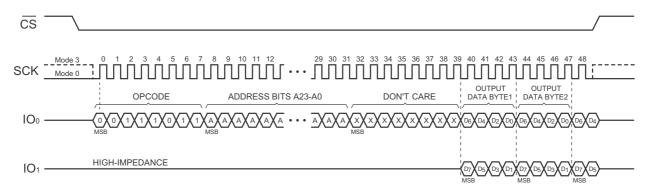
Figure 7. Dual-Output Read Array
