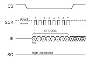
Figure 23. Erase/Program Resume Command Timing
