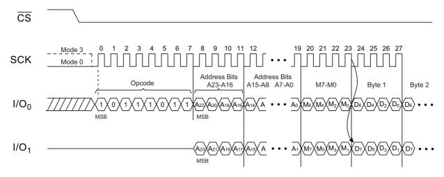
Figure 8. Dual-I/O Fast Read Array (Initial command or previous M5, M4 ≠ 1,0)
