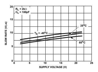
FIGURE 14. SLEW RATE vs SUPPLY VOLTAGE
