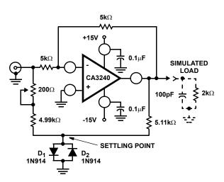
FIGURE 25C. TEST CIRCUIT (INVERTING) FIGURE 25. INPUT VOLTAGE vs SETTLING TIME
