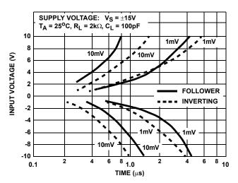
FIGURE 25A. SETTLING TIME vs INPUT VOLTAGE
