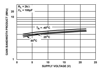
FIGURE 13. GAIN BANDWIDTH PRODUCT vs SUPPLY VOLT-AGE
