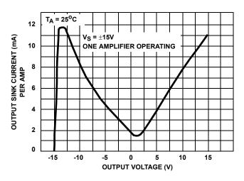
FIGURE 20. OUTPUT SINK CURRENT vs OUTPUT VOLTAGE
