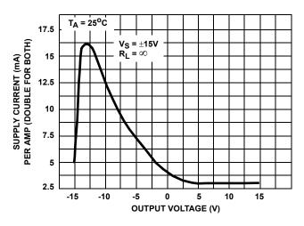
FIGURE 21. SUPPLY CURRENT vs OUTPUT VOLTAGE
