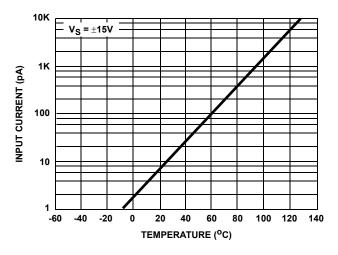
FIGURE 26. INPUT CURRENT vs TEMPERATURE
