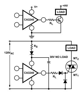
FIGURE 3. METHODS OF UTILIZING THE V<sub>CE (SAT)</sub> SINKING CURRENT CAPABILITY OF THE CA3240 SERIES
