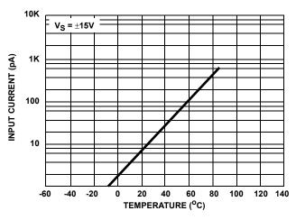
FIGURE 4. INPUT CURRENT vs TEMPERATURE
