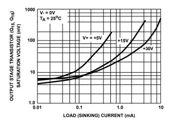
FIGURE 23. VOLTAGE ACROSS OUTPUT TRANSISTORS Q<sub>15</sub> AND Q<sub>16</sub> vs LOAD CURRENT
