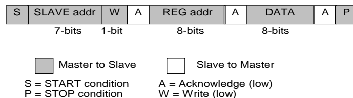
Figure 22: I2C byte write (SDA signal)
