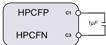
Figure 41. Charge pump flying capacitor
