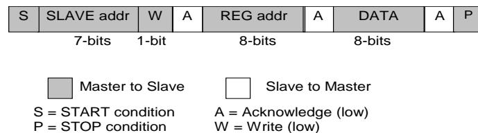
Figure 24: I 2 C Byte Write (SDA line)
