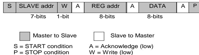
Figure 24: I 2 C Byte Write (SDA line)
