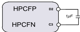
Figure 39: Charge Pump Flying Capacitor
