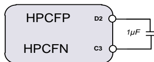
Figure 39: Charge Pump Flying Capacitor
