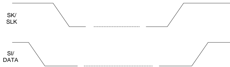
Figure 24: Timing of 2-WIRE START and STOP Condition
