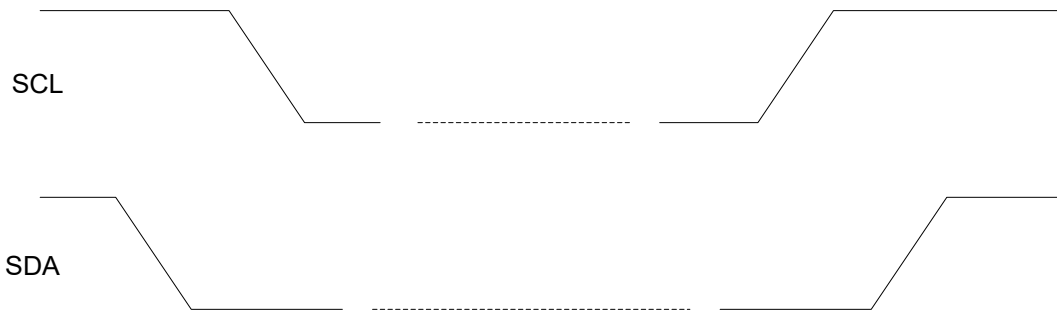
Figure 18: I 2 C START and STOP Condition Timing
