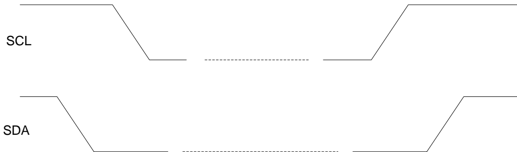
Figure 21: I 2 C START and STOP Condition Timing
