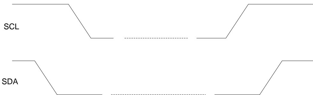
Figure 11: I 2 C START and STOP Condition Timing
