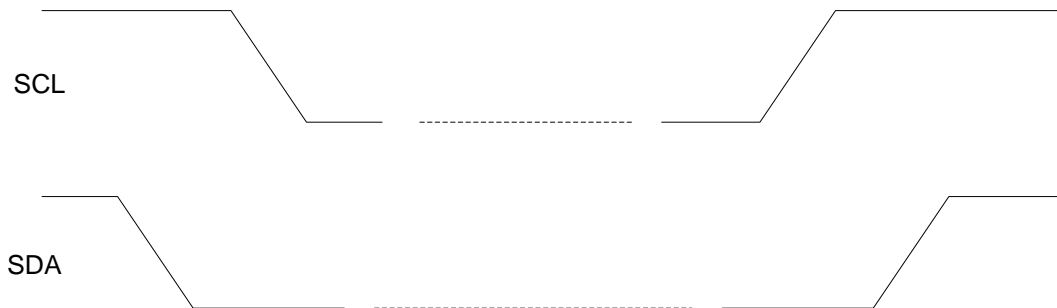
Figure 9: I 2 C START and STOP Condition Timing
