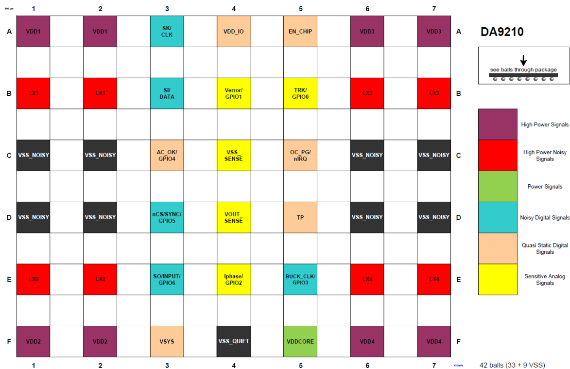
Figure 3: Connection Diagram (42 VFBGA)
