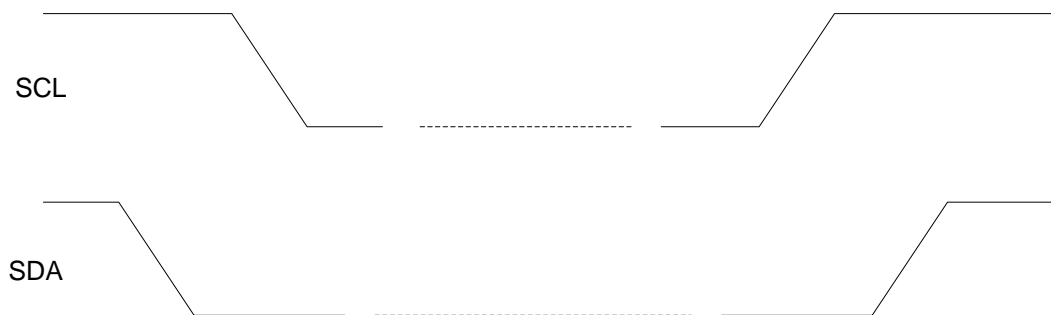
Figure 42: Timing of 2-WIRE START and STOP Condition
