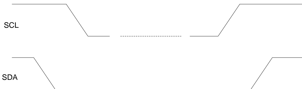
Figure 23: Timing of 2-WIRE START and STOP Condition
