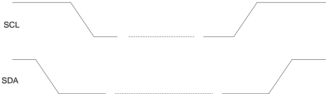
Figure 17: I 2 C START and STOP Condition Timing
