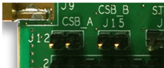
Figure 80. Jumpers for Serial Programming Connections
