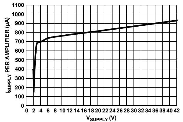
FIGURE 26. SUPPLY CURRENT vs SUPPLY VOLTAGE
