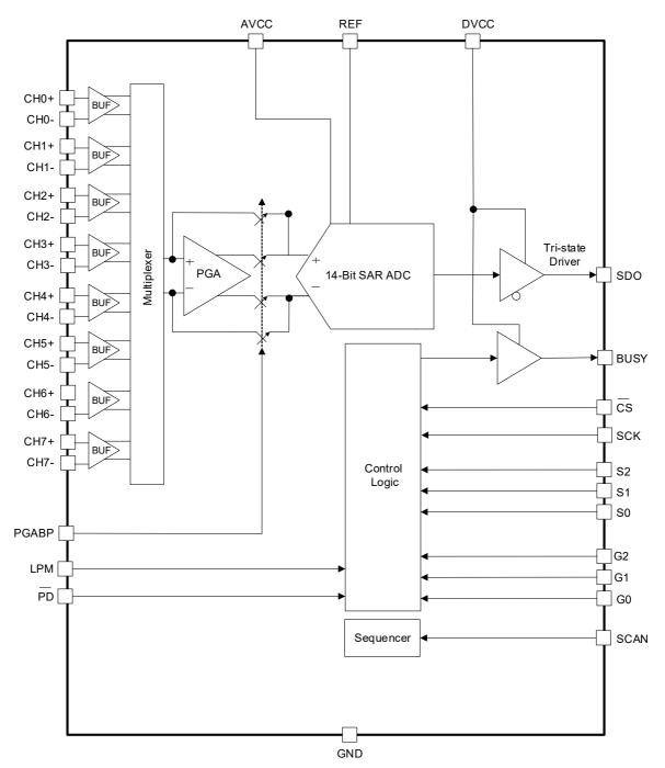
Figure 4. Block Diagram
