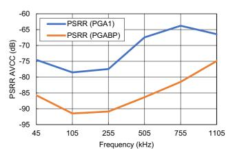
Figure 51. PSRR vs Frequency- AVCC
