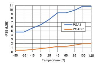
Figure 50. -Full-Scale Error vs Temperature
