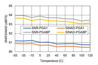
Figure 117. SNR and SINAD vs Temperature
