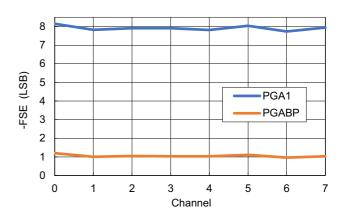
Figure 92. -Full-Scale Error vs Channel
