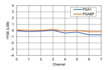
Figure 46. +Full-Scale Error vs Channel
