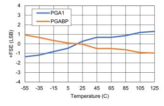
Figure 90. +Full-Scale Error vs Temperature
