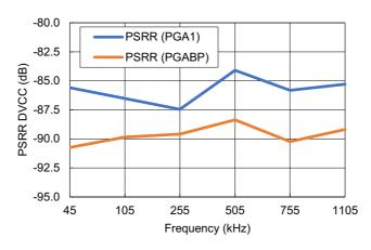
Figure 52. PSRR vs Frequency- DVCC
