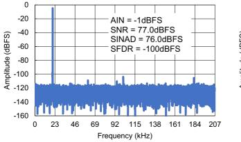
Figure 63. 32k FFT - 20.3kHz, PGA = 2
