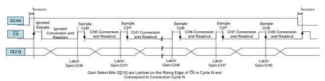
Figure 123. SCAN and Gain Select Timing Diagram - Low Power Mode
