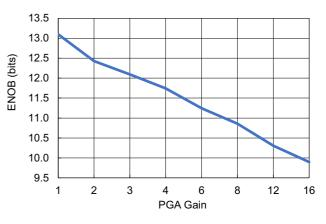
Figure 115. ENOB vs PGA Gain
