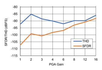
Figure 116. THD and SFDR vs PGA Gain
