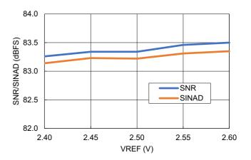
Figure 80. SNR and SINAD vs VREF
