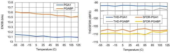
Figure 106. ENOB vs Temperature
