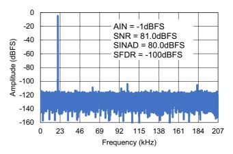
Figure 62. 32k FFT - 20.3kHz, PGA = 1
