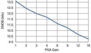
Figure 30. ENOB vs PGA Gain
