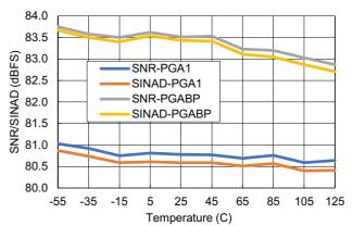
Figure 74. SNR and SINAD vs Temperature
