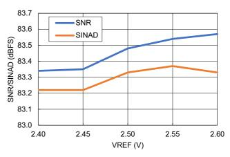
Figure 37. SNR and SINAD vs VREF
