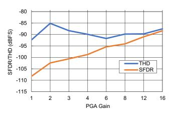
Figure 104. THD and SFDR vs PGA Gain
