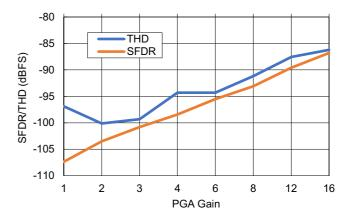
Figure 29. THD and SFDR vs PGA Gain
