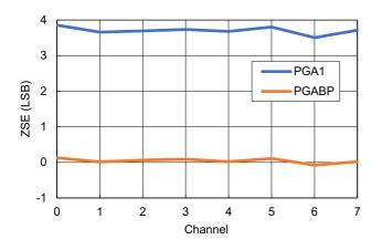
Figure 87. Zero-Scale Error vs Channel
