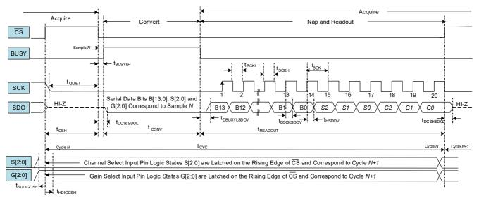
Note: Bits S2, S1, S0, G2, G1, and G0 are optional and not required. For maximum sample rate, do not provide additional clocks for these bits.
