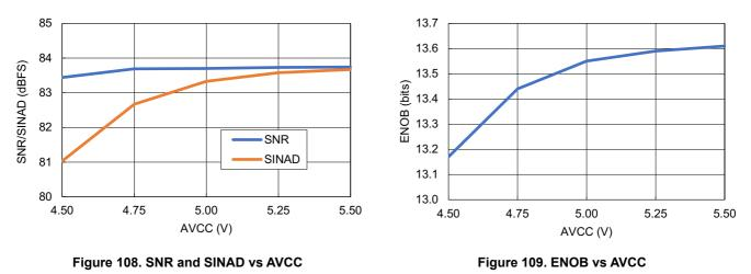
Unless otherwise noted,  $AV_{CC} = 5.0V$ ;  $DV_{CC} = 2.5V$ , REF = 2.5V, GND = 0V, PGA Bypassed, LPM =  $DV_{CC}$ ,  $f_{SAMP} = 684.932$ ksps,  $F_{IN} = 20.3$ kHz,  $A_{IN} = -7$ dBFS, CH(0:7)- connected to  $V_{REF}/2$ ;  $T_A = 25^{\circ}$ C.
