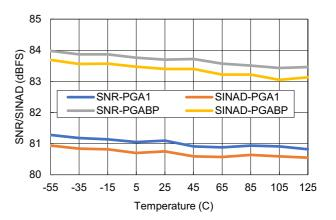
Figure 105. SNR and SINAD vs Temperature
