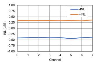
Figure 15. INL vs Channel
