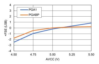
Figure 45. +Full-Scale Error vs AVCC
