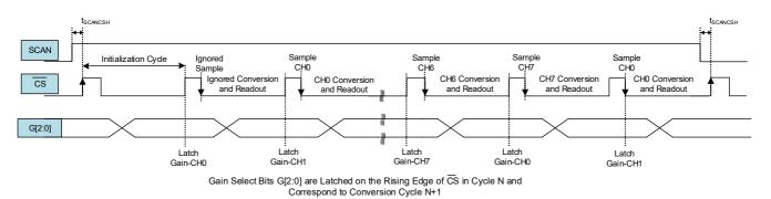
Figure 7. SCAN Timing Diagram - Normal Mode
