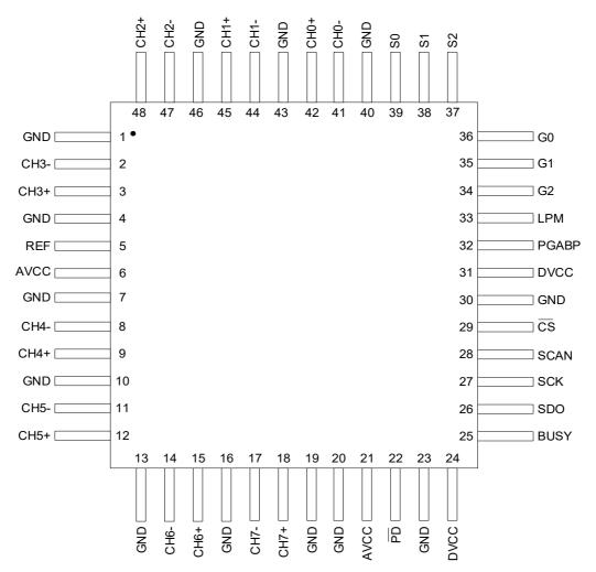
Figure 5. Pin Assignments - Top View
