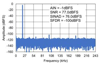
Figure 21. 32k FFT - 20.3kHz, PGA = 4
