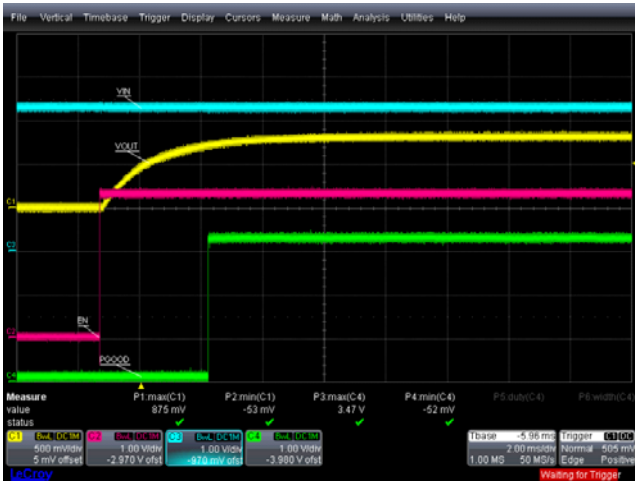
FIGURE 23. POWER-ON AND POWER-OFF, EN = 0 TO 1, +25°C, VIN = 6V, VOUT = 0.8V, IOUT = 0.5A, PGOOD TURN-ON
