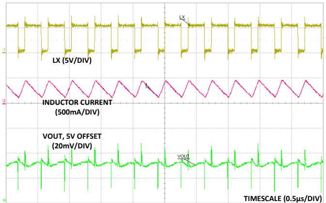
FIGURE 12. PWM MODE OPERATION ( V_{IN} = 3.6\text{V} , V_{OUT} = 5\text{V} , 200mA LOAD)
