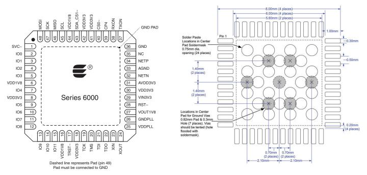
Figure 3. 6K IC Pin Configuration
