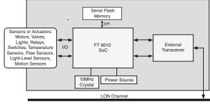
Figure 9. Typical Neuron 6050-based Device
