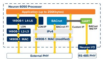
Figure 1. Neuron 6050 Firmware Protocol Stacks
