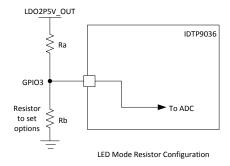
Figure 8 P9036B LED Resistor Options.
