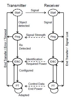
Figure 6 System State Machine Diagram
