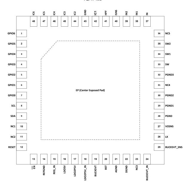
Figure 2 P9036B Pin Configuration (NTG48 TQFN-48L 6.0 mm x 6.0 mm x 0.75 mm, 0.4mm pitch)
