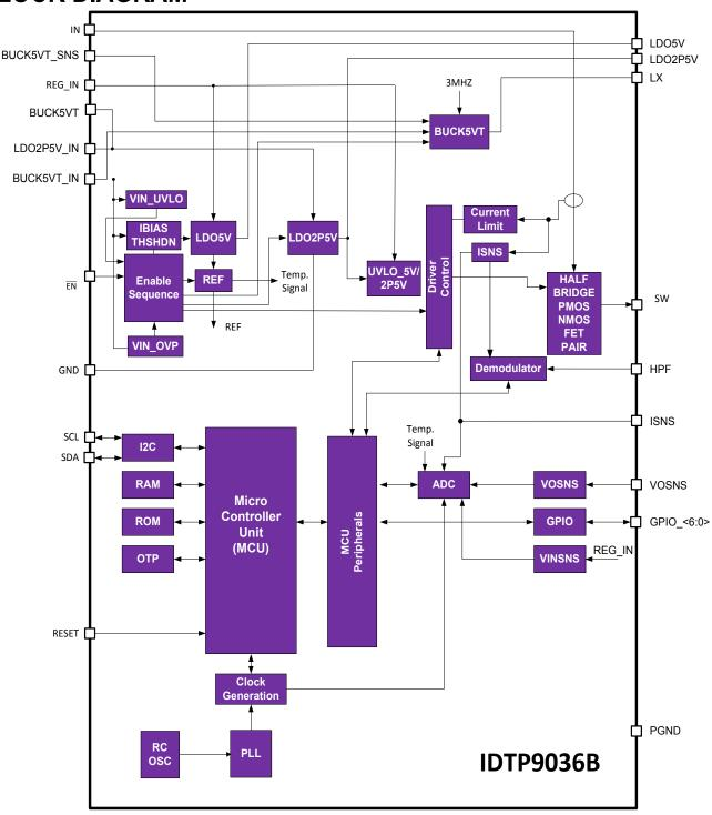
Figure 4. P9036B Internal Functional Block Diagram
