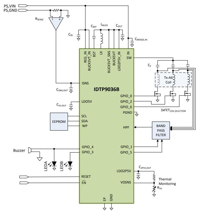
Figure 1. P9036B Simplified Application Schematic
