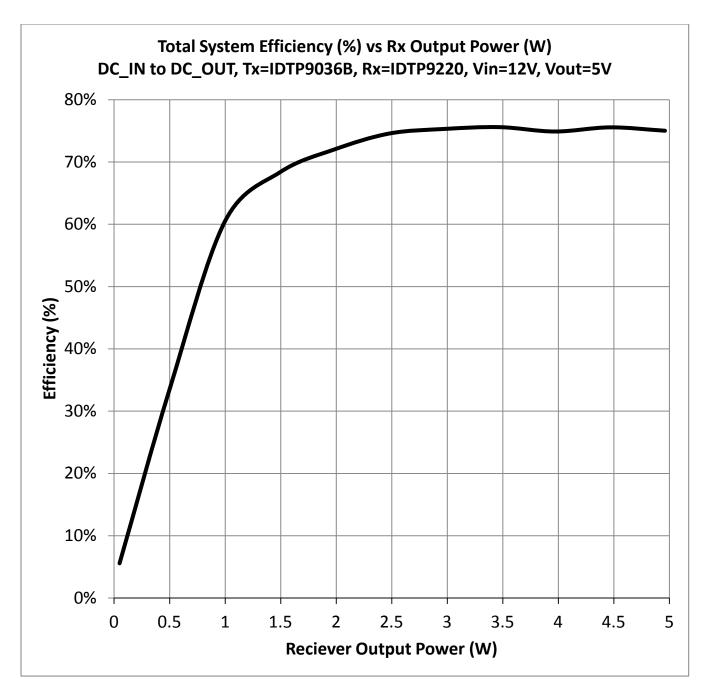
Figure 3. Efficiency vs. RX Output Power
