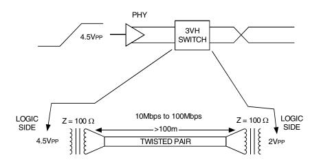
Fast Ethernet Data Switching (LAN Switch)
