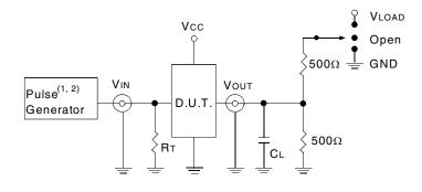
Test Circuits for All Outputs
