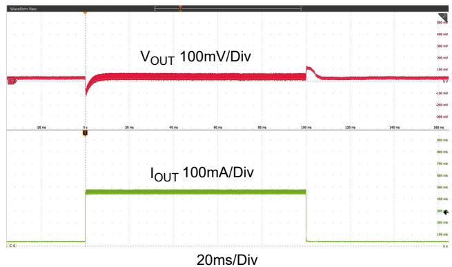
Figure 19. Load Transient (45mA-450mA)
