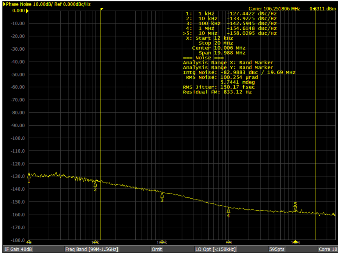
Figure 5. Phase Noise of 106.25MHz Output in Clock Generator Mode
