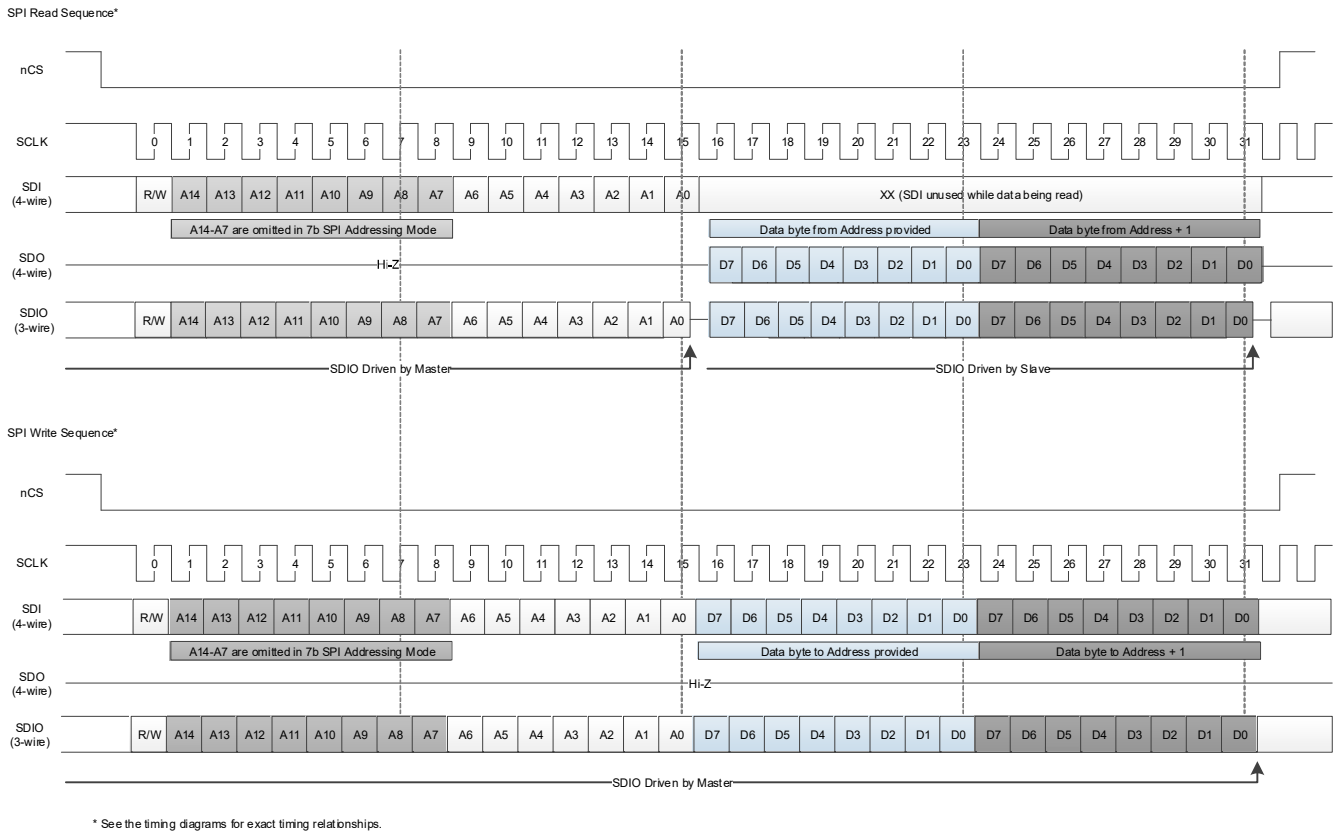
Figure 21. SPI Sequencing
