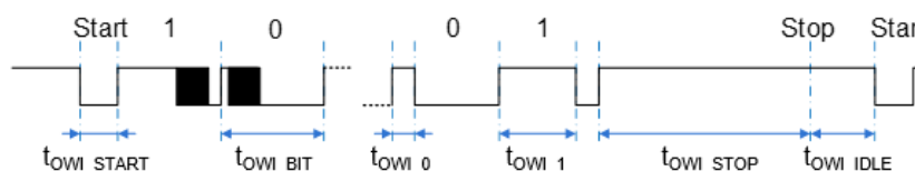
Figure 21. OWI Timing Diagram
