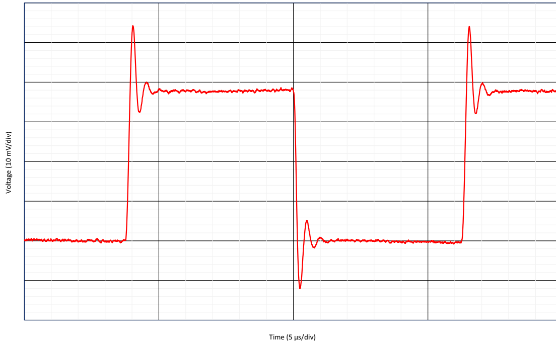
Figure 117. Small Signal Non-Inverting Step Response G = -1 V/V, R_L = 50 k \Omega , C_L = 60 pF, BW = 2 MHz
