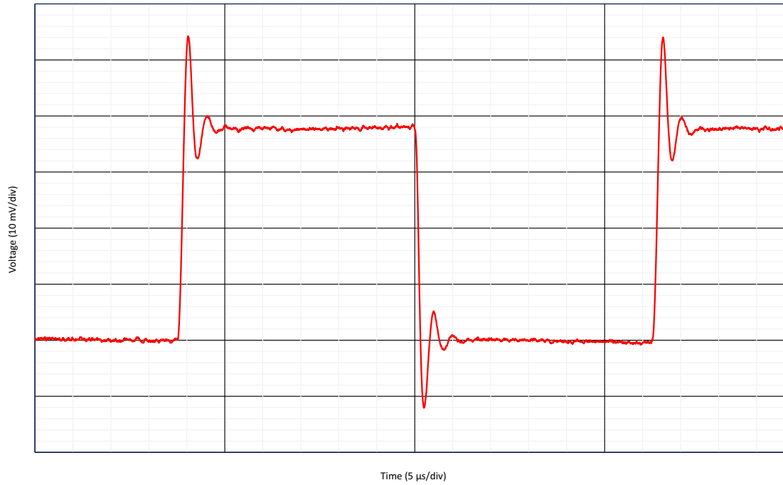
Figure 114: Small Signal Non-Inverting Step Response G = -1 \text{ V/V} , R_L = 50 \text{ k}\Omega , C_L = 60 \text{ pF} , BW = 2 \text{ MHz}
