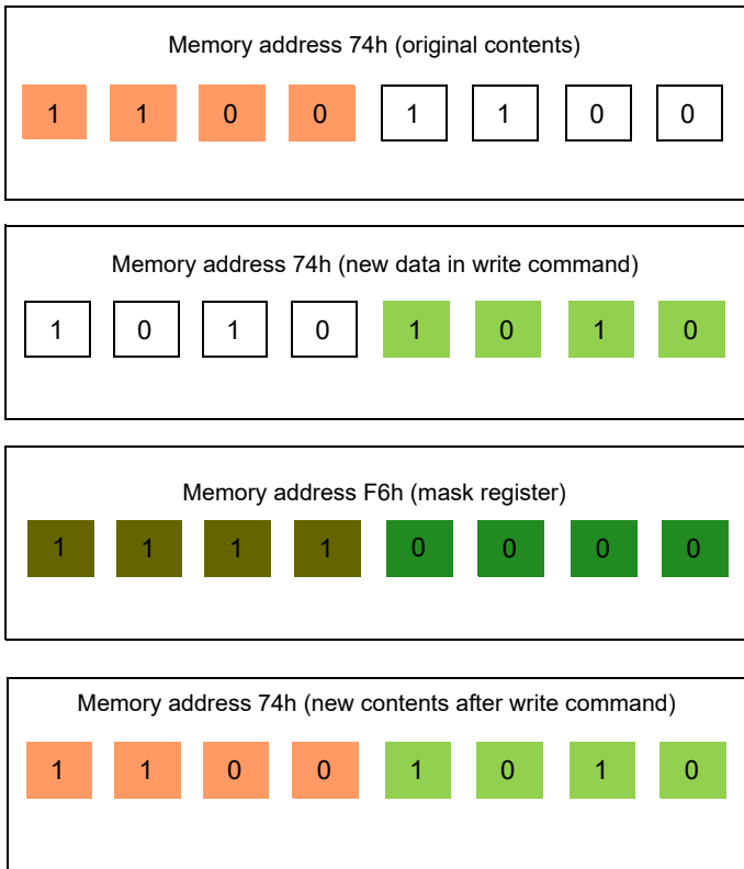
Figure 162. Example of I 2 C Byte Write Bit Masking
