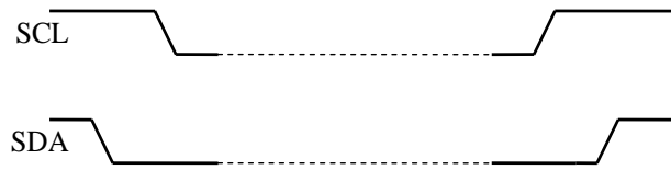
Figure 13. I 2 C Start and Stop Conditions
