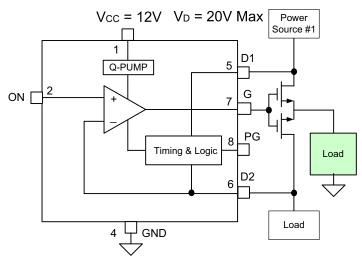
SLG55026 For N-MOSFETS with  $8V < V_{GD2} < 16V$
