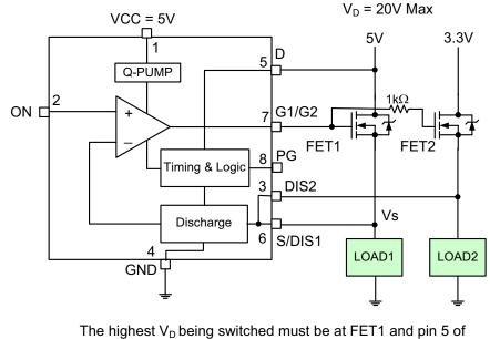
The highest V<sub>D</sub> being switched must be at FET1 and pin 5 of the SLG55221 and SLG55220
