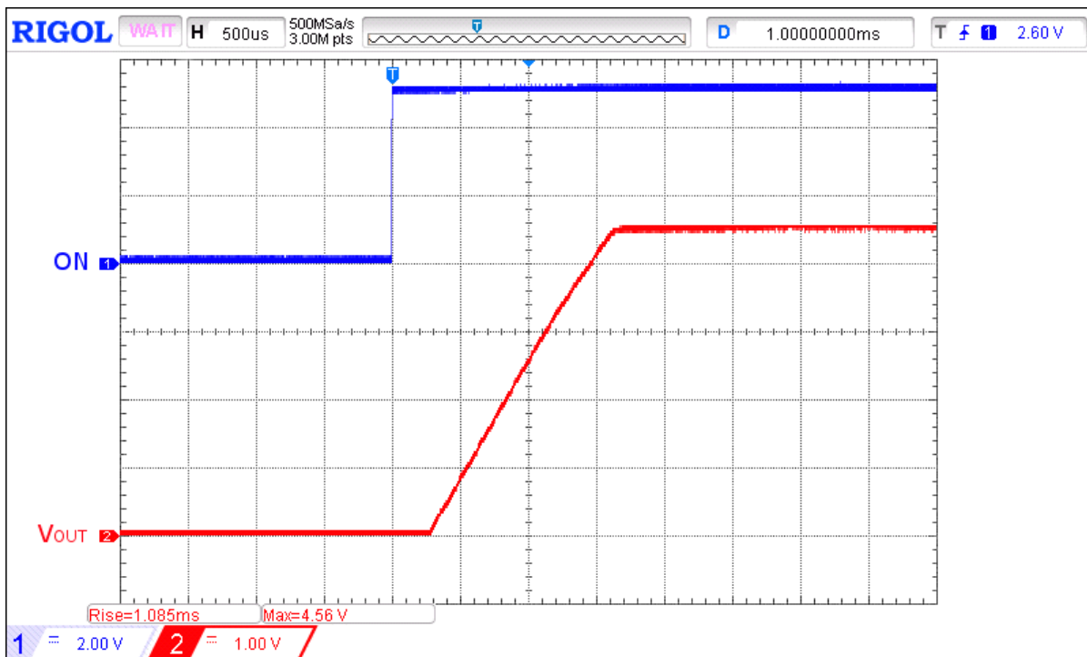
Figure 2. Typical Turn ON operation waveform for V_{IN} = 4.5\text{ V} , C_{SLEW} = 10\text{ nF} , C_{LOAD} = 10\text{ }\mu\text{F} , R_{LOAD} = 100\text{ }\Omega
