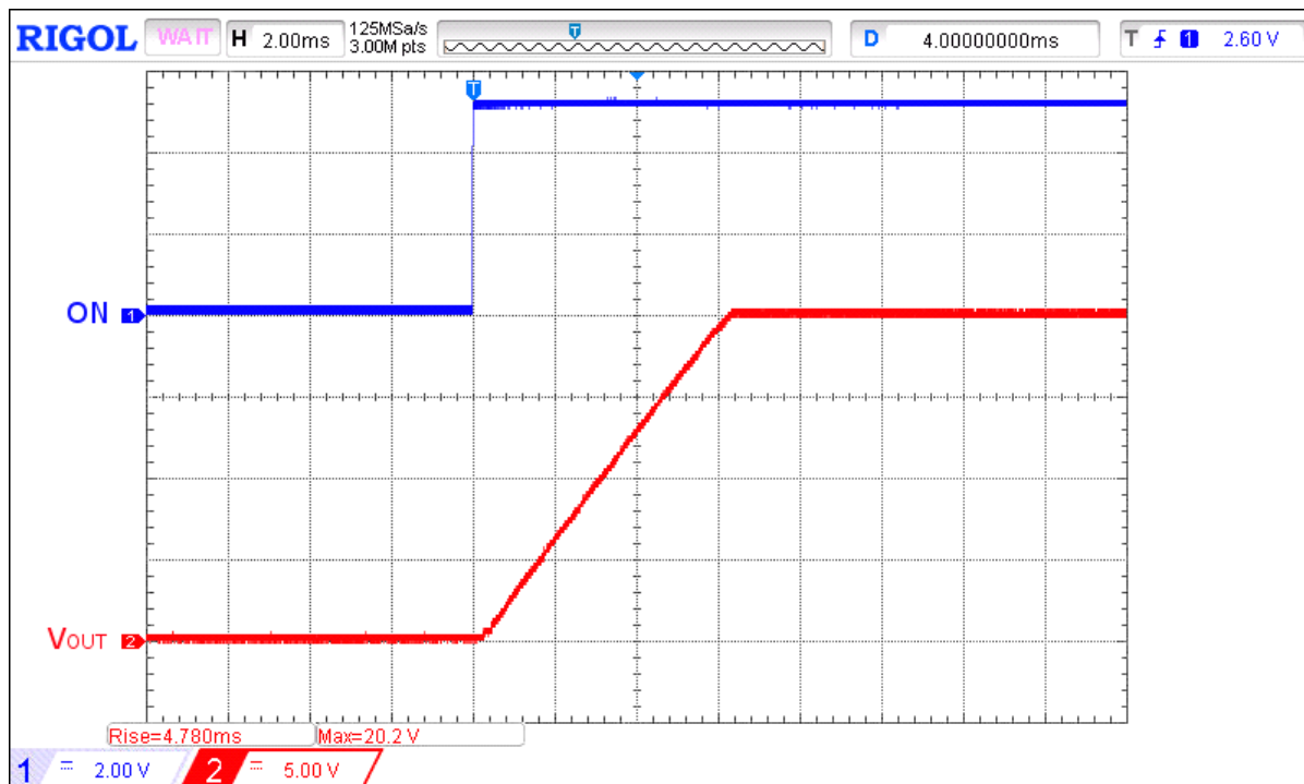
Figure 8. Typical Turn ON operation waveform for V_{IN} = 20\text{ V} , C_{SLEW} = 10\text{ nF} , C_{LOAD} = 10\text{ }\mu\text{F} , R_{LOAD} = 100\text{ }\Omega
