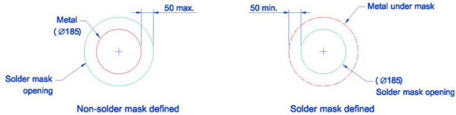
Solder mask detail (not to scale)
