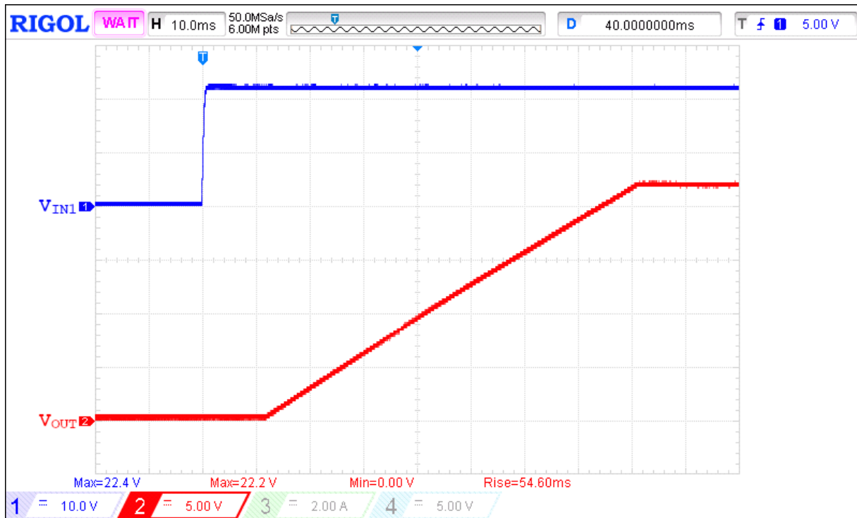
Figure 3. Typical Turn ON operation waveform for V_{IN1} = 22\text{ V} , C_{SS} = 220\text{ nF} , R_{LOAD} = 100\ \Omega , C_{LOAD} = 2\ \mu\text{F}
