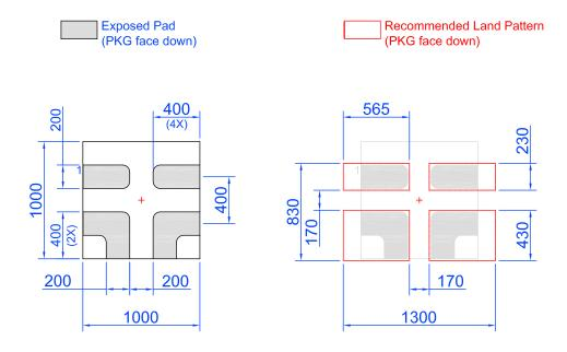
Note: All dimensions shown in micrometers (µm)
