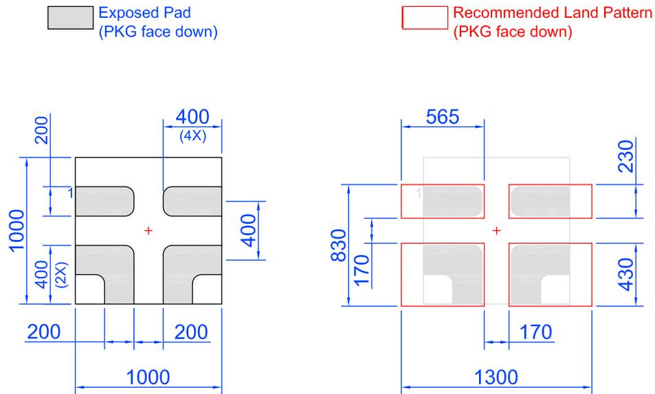
Note: All dimensions shown in micrometers (μm)
