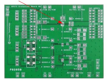
Figure 1. SLG59M1655V Evaluation Board.
