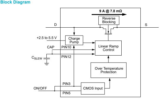
An Ultra-small, 7.8 m $\Omega$ , 9 A, Single-channel Load Switch with Reverse-current Blocking
