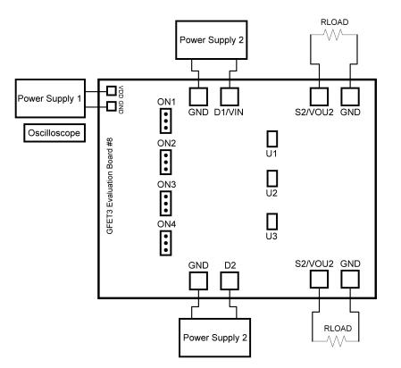
Figure 3. Typical connections for GFET3 Evaluation.
