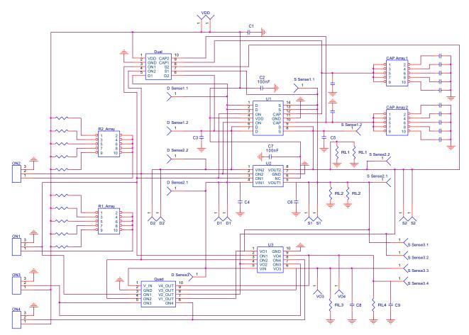
Figure 2. SLG59M1655V Evaluation Board Connection Circuit.
