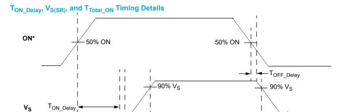
Note: \* Rise and Fall times of the ON signal are 100 ns
