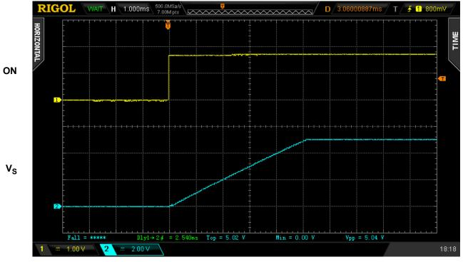
Figure 2. Typical Turn ON operation waveform for  $V_{DD}$  =  $V_{D}$  = 5 V,  $C_{SLEW}$  = 12 nF,  $C_{LOAD}$  = 10  $\mu$ F,  $R_{LOAD}$  = 20  $\Omega$
