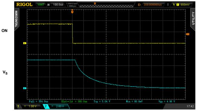
Figure 4. Typical Turn OFF operation waveform for  $V_{DD}$  =  $V_{D}$  = 5 V,  $C_{SLEW}$  = 4 nF,  $C_{LOAD}$  = 10  $\mu$ F,  $R_{LOAD}$  = 20  $\Omega$
