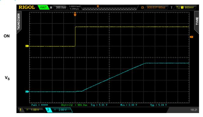
Figure 1. Typical Turn ON operation waveform for  $V_{DD}$  =  $V_{D}$  = 5 V,  $C_{SLEW}$  = 4 nF,  $C_{LOAD}$  = 10  $\mu$ F,  $R_{LOAD}$  = 20  $\Omega$
