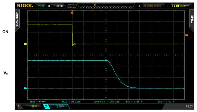
Figure 3. Typical Turn OFF operation waveform for  $V_{DD}$  =  $V_D$  = 5 V,  $C_{SLEW}$  = 4 nF, no  $C_{LOAD}$ ,  $R_{LOAD}$  = 20  $\Omega$
