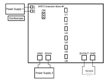
Figure 7. Typical connections for GreenFET Evaluation
