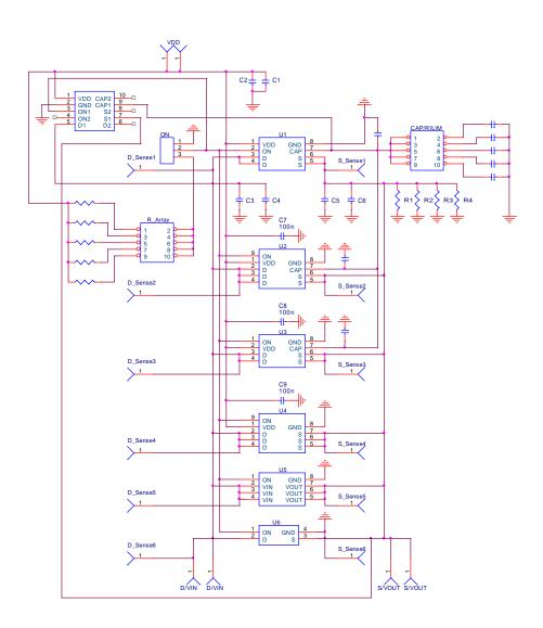
Figure 6. SLG59M1657V Evaluation Board Connection Circuit
