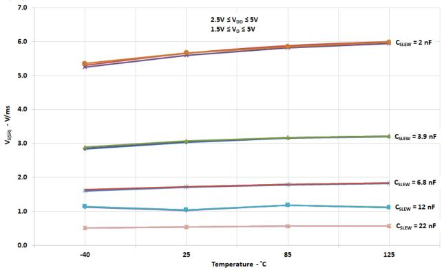
$\mathbf{T}_{Total~ON}$  vs.  $\mathbf{C}_{SLEW},\,\mathbf{V}_{D},\,\mathbf{V}_{DD},$  and Temperature
