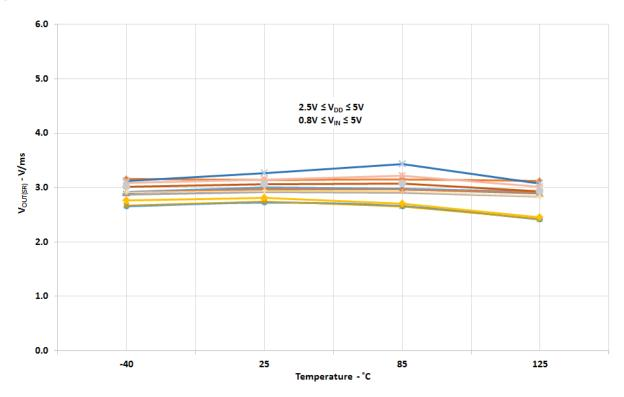
$T_{Total\ ON}$  vs. Temperature,  $V_{DD},$  and  $V_{IN}$
