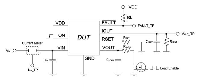
Figure 7. Test setup Application Diagram
