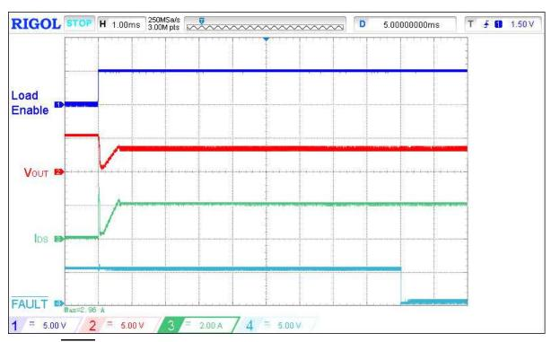
Figure 9. Typical  $\overline{FAULT}$  assertion waveform for  $V_{DD} = V_{IN} = 5$  V,  $C_{LOAD} = 10$   $\mu$ F,  $I_{ACL} = 2$  A,  $R_{SET} = 40$  k $\Omega$ , switch in 2  $\Omega$  load
