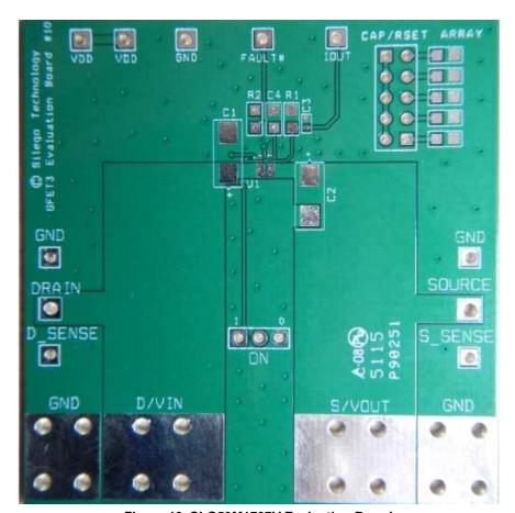
Figure 13. SLG59M1707V Evaluation Board
