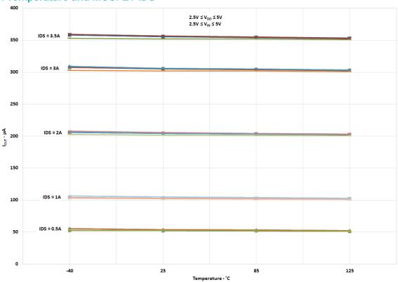
**I<sub>OUT</sub> vs. MOSFET IDS and Temperature**
