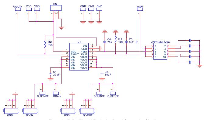
Figure 14. SLG59M1707V Evaluation Board Connection Circuit
