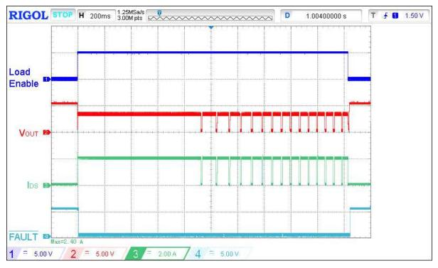
Figure 8. Typical ACL operation waveform for  $V_{DD}$  =  $V_{IN}$  = 5 V,  $C_{LOAD}$  = 10  $\mu$ F,  $I_{DS}$  = 2 A,  $R_{SET}$  = 40  $k\Omega$
