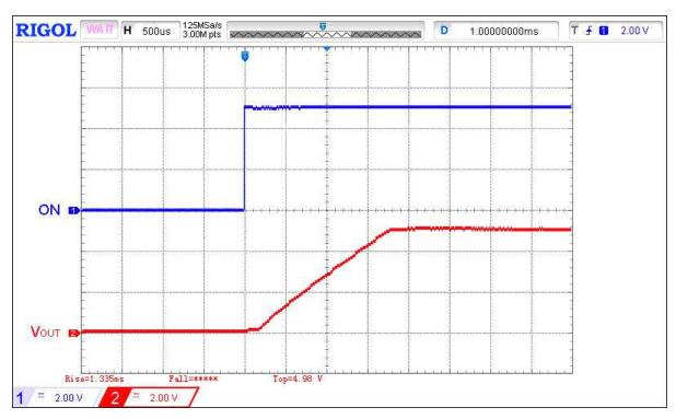
Figure 1. Typical Turn ON operation waveform for  $V_{DD}$  =  $V_{IN}$  = 5 V,  $C_{LOAD}$  = 10  $\mu$ F,  $R_{LOAD}$  = 20  $\Omega$
