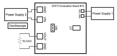
Figure 15. SLG59M1707V Evaluation Board Connection Circuit
