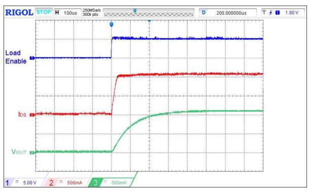
Figure 11. Typical  $I_{OUT}$  response time waveform for  $V_{DD}$  =  $V_{IN}$  = 5 V,  $C_{LOAD}$  = 10  $\mu$ F,  $R_{LOAD}$  = 5  $\Omega$ ,  $C_{IOUT}$  = 0.01  $\mu$ F,  $R_{IOUT}$  = 10  $k\Omega$ , Load Step 0 A to 1 A
