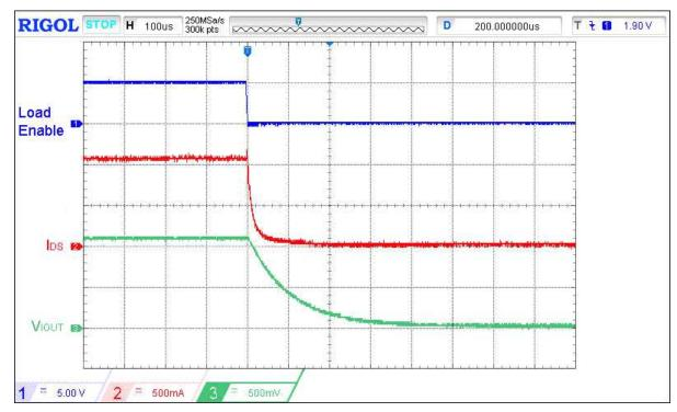
Figure 12. Typical  $I_{OUT}$  response time waveform for  $V_{DD}$  =  $V_{IN}$  = 5 V,  $C_{LOAD}$  = 10  $\mu$ F,  $R_{LOAD}$  = 5  $\Omega$ ,  $C_{IOUT}$  = 0.01  $\mu$ F,  $R_{IOUT}$  = 10  $k\Omega$ , Load Step 1 A to 0 A
