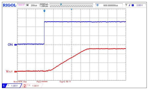
Figure 2. Typical Turn ON operation waveform for  $V_{DD}$  =  $V_{IN}$  = 2.5 V,  $C_{LOAD}$  = 10  $\mu$ F,  $R_{LOAD}$  = 20  $\Omega$
