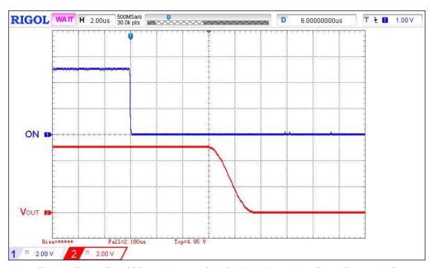
Figure 3. Typical Turn OFF operation waveform for  $V_{DD}$  =  $V_{IN}$  = 5 V, no  $C_{LOAD}$ ,  $R_{LOAD}$  = 20  $\Omega$
