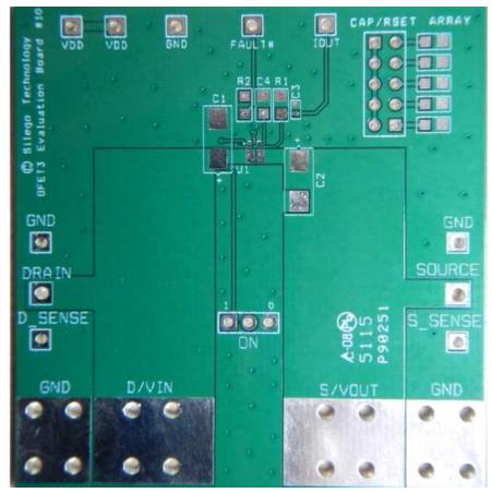
Figure 8. SLG59M1717V Evaluation Board
