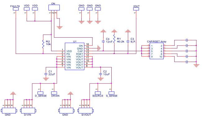
Figure 9. SLG59M1717V Evaluation Board Connection Circuit
