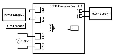
Figure 10. SLG59M1717V Evaluation Board Connection Circuit
