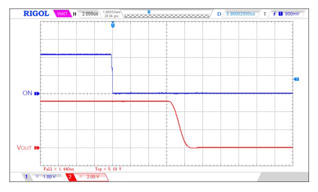
Figure 3. Typical Turn OFF operation waveform for  $V_{DD}$  =  $V_D$  = 5 V,  $C_{SLEW}$  = 12 nF,  $R_{LOAD}$  = 20  $\Omega$ , no  $C_{LOAD}$
