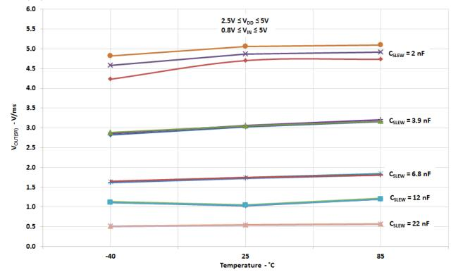
$V_{OUT(SR)}$  vs. C<sub>SLEW</sub>, V<sub>IN</sub>, V<sub>DD</sub>, and Temperature
