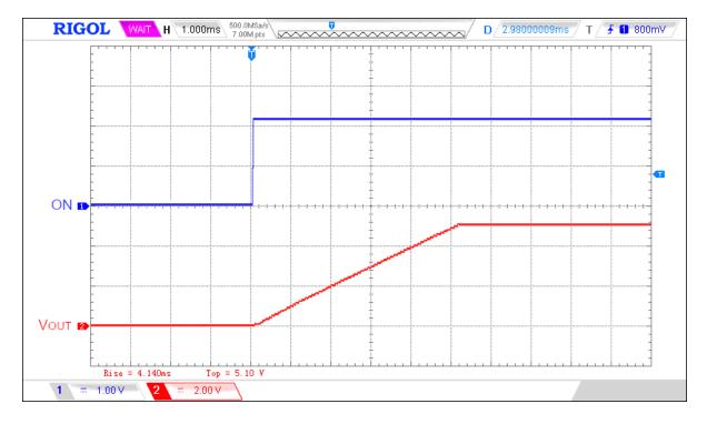
Figure 1. Typical Turn ON operation waveform for  $V_{DD}$  =  $V_D$  = 5 V,  $C_{SLEW}$  = 12 nF,  $C_{LOAD}$  = 10 µF,  $R_{LOAD}$  = 20  $\Omega$
