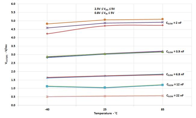
$V_{OUT(SR)}$  vs. C<sub>SLEW</sub>, V<sub>IN</sub>, V<sub>DD</sub>, and Temperature
