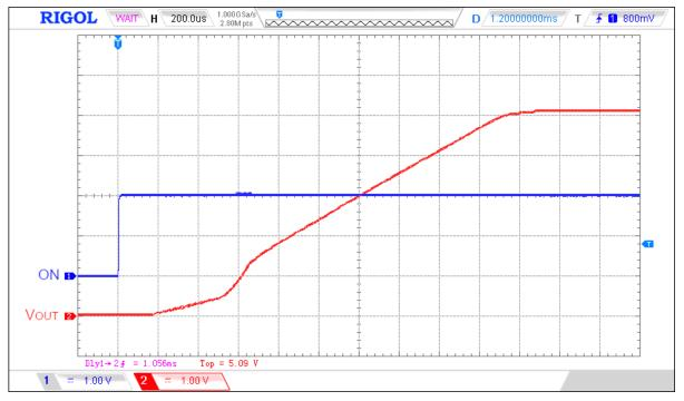
Figure 6. A SLG59M1717V with C<sub>SLEW</sub> set to 4nF and 470µF for C<sub>LOAD</sub>. C<sub>LOAD</sub>-to-C<sub>SLEW</sub> ratio is greater than 33,600. Note that the internal SCL monitor's been triggered and V<sub>OUT(SR)</sub> is reduced until V<sub>OUT</sub> reaches ~0.25V.
