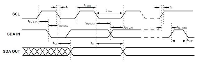
Figure2. I2C Serial General Timing
