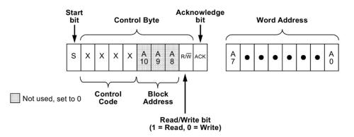
Figure 1. I2C Basic Command Structure
