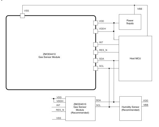
Figure 3. Application Circuit
