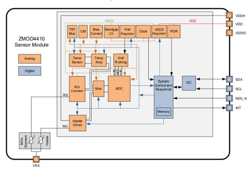
Figure 2. Block Diagram
