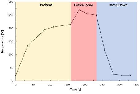
Figure 14. Typical Solder Profile
