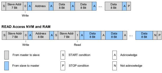
Figure 15. I<sup>2</sup>C Data Transmission Protocol
