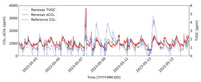
Figure 8. Typical Graph of CO<sub>2</sub> Estimation in an Application
