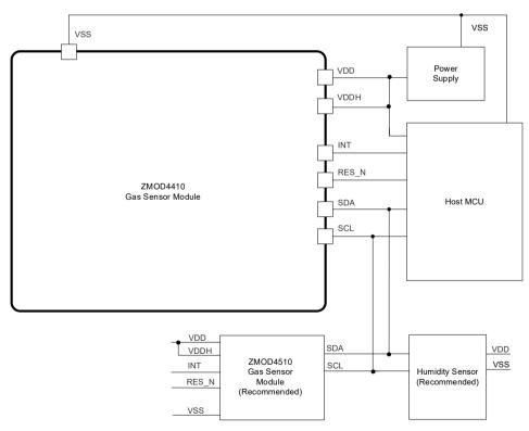
Figure 3. Application Circuit
