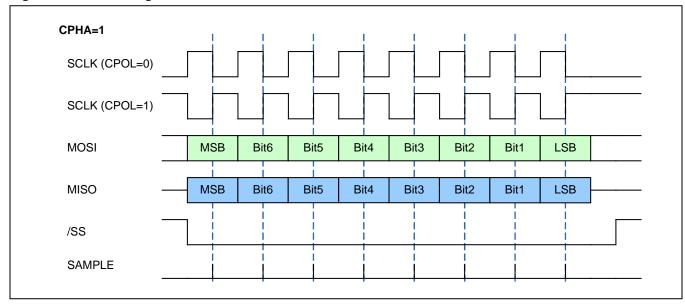
Figure 3.4 SPI Configuration CPHA=1
