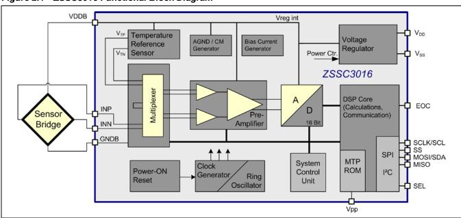
Figure 2.1 ZSSC3016 Functional Block Diagram
