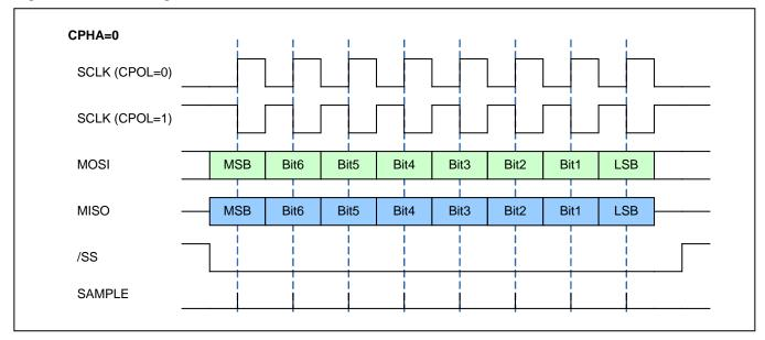
Figure 3.3 SPI Configuration CPHA=0
