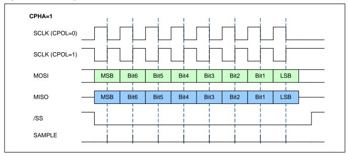
In SPI mode, each command except NOP is started as shown in Figure 3.5. After the execution of a command (busy = 0), the expected data can be read as illustrated in Figure 3.6 or if no data are returned by the command, the next command can be sent. The status can be read at any time with the NOP command (see Figure 3.7).
