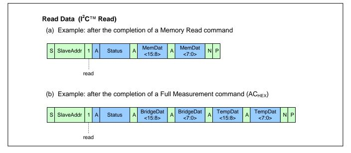
All mandatory I<sup>2</sup>C-bus protocol features are implemented. Optional features like clock stretching, 10-bit slave address, etc., are not supported by the ZSSC3027's interface.
