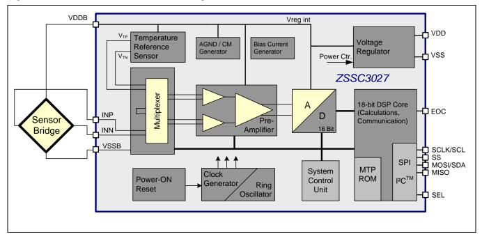
Figure 2.1 ZSSC3027 Functional Block Diagram
