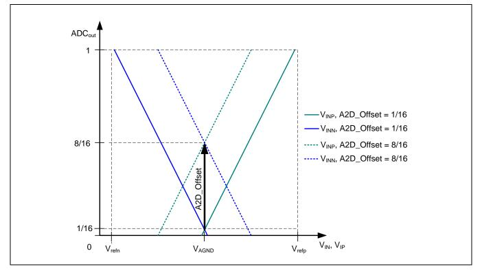
Table 2.8 ADC Offset Settings for the Measurement Configuration Register BM\_config
